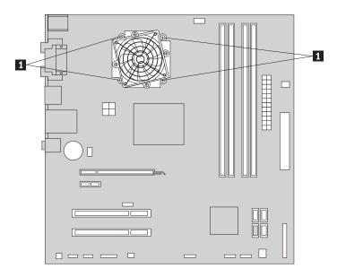
Figure 20. Removing the heat sink and fan assembly
